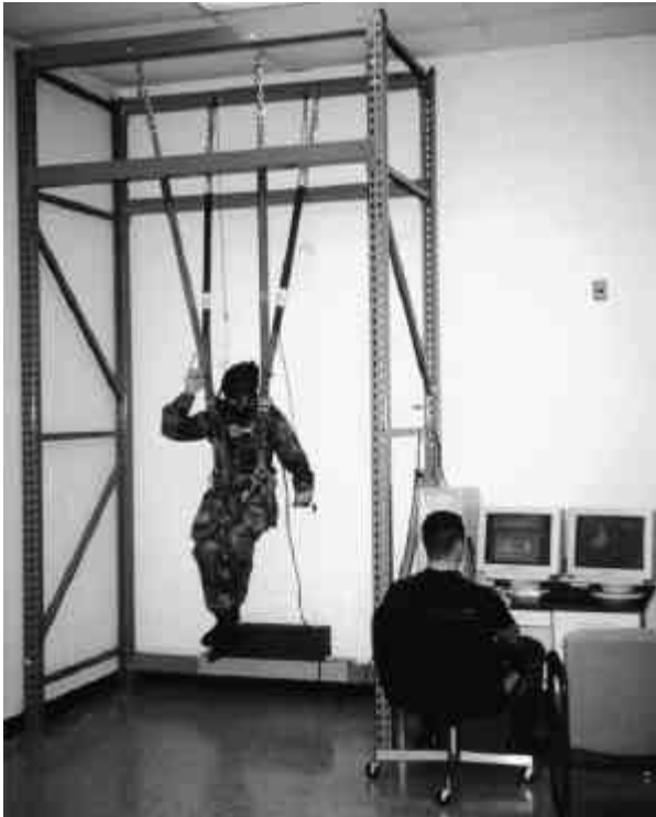
Figure 11. VR Parachute Simulator Suspension Frame
