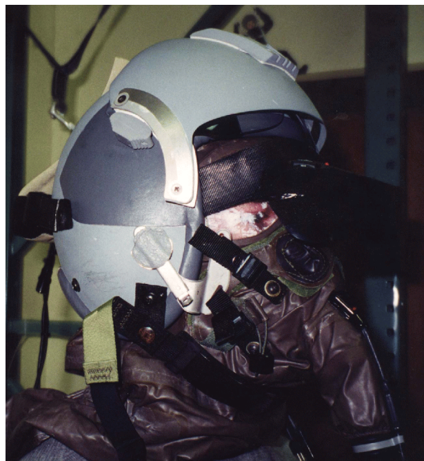
Figure 2. AERPS Under HMD and Dual Visor Hemet with Head Tracker
