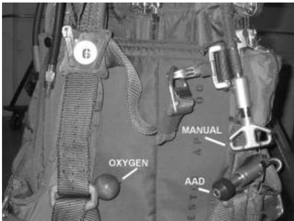
Figure 7. BA18 Manual, AAD, and O 2 Emergency Ripcords
